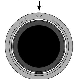
**CAUTION: The dial should not be pushed in until the combination has been dialed and the dial returned to zero at the opening index.**
