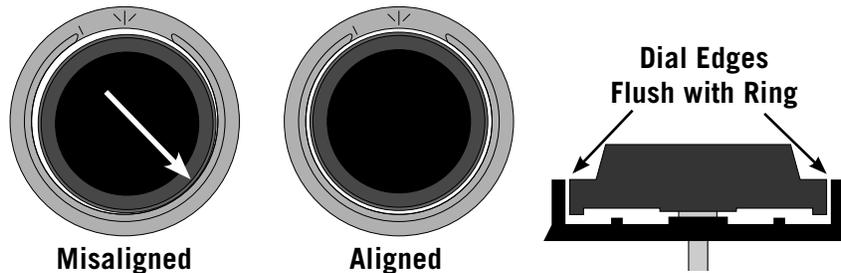
*Note that the small gap between the dial and ring is uneven when the dial ring is misaligned (see arrow above), but is even when the dial ring is properly aligned. The center of a properly aligned dial ring is in perfect alignment with the center of the spindle hole in the drive cam.*
