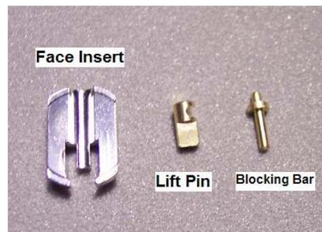
The Blocking Bar is inserted first. It lies horizontally across the face of the plug. The Lift Pin fits vertically over the Lifting Bar.
