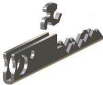
The standard BiLock key is made from Nickel Silver and has as a double row of cuts that are made prior to final forming. The key assembly includes the key blade, a Trigger, and the three piece key head.
