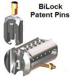
Notice how the Blocking Bar sits in line with the Side Bar holes when it is the rest (locked) position.
